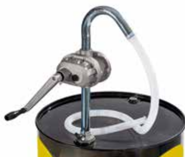
Art. 027-3710-000 Aluminium rotary barrel pump H.D. Delivery capacity 80 l/min With suction hose and 2" adaptor for the connection to the barrels Delivery hose 1,80 m lenght Suitable for diesel, lubricants and gasoline transfer
