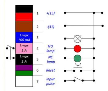
Lamp linked to 3 contact is **fixed on** during working time or when reset button has been pushed and **lamps** when there's an alarm
